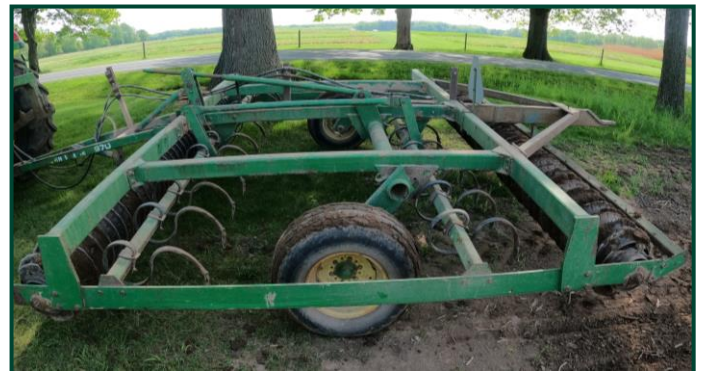
A disc and cultipacker can help improve seedbeds. Photo courtesy of Fahimeh Baziari.
